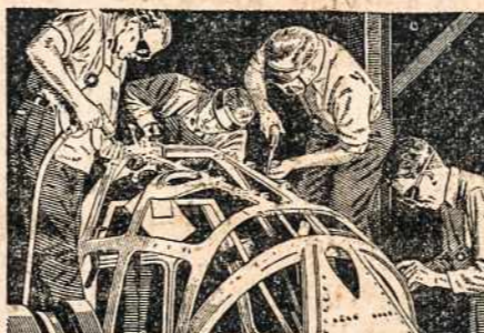
At Willow Run the top section of the bombardier's enclosure, formerly made in 13 hand-formed pieces - is now made in only 3 parts - saving 30 hours in the construction time of each bomber.
